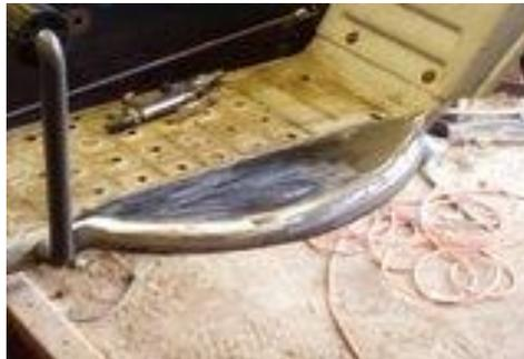
Here ya go. The deck pieces welded in place. Nothing left now but some slight bondo to clean it up and weld the shifter hole closed in the right fender. Then bondo it, then finish the body work, paint it, the wiring and motor. (Another Big INDIAN) 🤪
