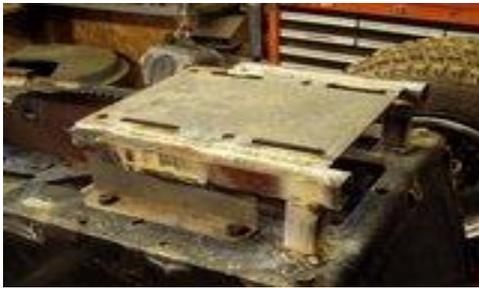
Here is a better view of what I have done. You can see at the rear where I added an upright support with same size tubing. Fender will bolt down on top of all this and seat will bolt into the slotted groove where it gives you the ability to slide the seat forward or backwards the original amount. ALL legal and great for fine tuning the handling of your mower. Fenders will still bolt into the original holes in the running boards giving the appearance they haven't been moved.
