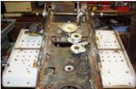
Here is an overall view of rear axle in place, with tranny pulley and clutch and guides in place. Also, notice the center of the running board rod is cut out as described in earlier details. This gives wide open access to everything.
