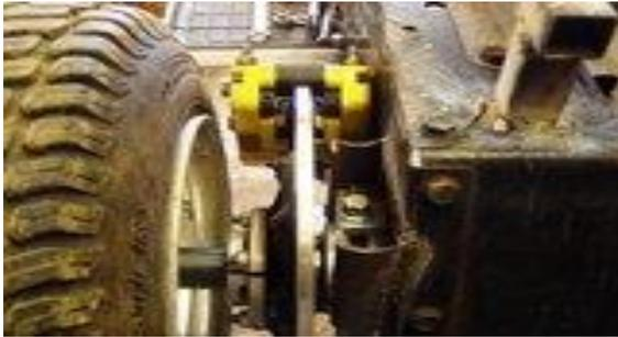
Here you can see the clearance between caliper and tire. Tire 19 inches from center of frame. That's the outer sidewall.
