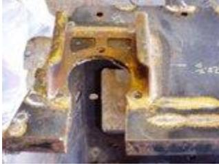
Here you can see where I have finally come back and cut the whole and slot for the rear axle. Doing it this way allows me to unbolt the cassettes and simply drop the whole axle out the bottom.
