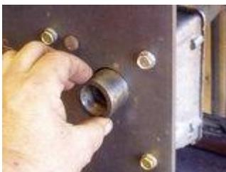
Here you see that I have mounted a tranny lower case. Then you slip the plate bushing into the the hole which self aligns on the input shaft.
