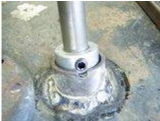
Here is the lower steering column support and bearing welded in. Notice in the pictures how it fits right in the pocket where the oem parts were. you will also notice how I use 5/8 lock collars one on top of lower bearing, and one on the bottom of upper bearing. I use a grinder and put a small notch so I can get to set screw.
