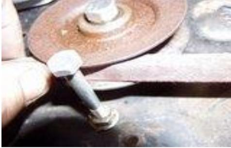
Now notice with my finger slightly pushing on belt, it sits deeper. So as you can see, it is simply there to keep belt from whipping back and forth. The guide on this pulley is not as the others. I drilled a hole, tapped it for standard thread, and ran a flanged nut on a 1/4 inch bolt. Screw it into the frame and the flange nut is the jam nut to keep it from backing out.
