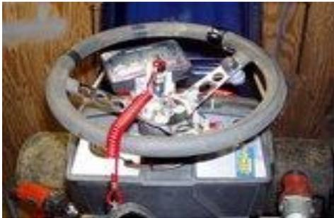
Here is the throttle setup ast the carbs. I use a throttle linkage kit from E.C. I believe the part number is 1k-122. I do modify it just a bit, but each application will be different.
