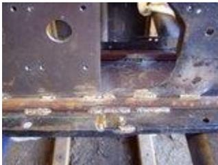
Ok here you see where the E.C. Distributing tranny plate butts right up against the front sub frame. ALSO it goes in the tunnel and sets on top of the frame rail supports. You can bolt or weld it in I choose to weld it then it becomes a part of the frame and helps stiffen it.
