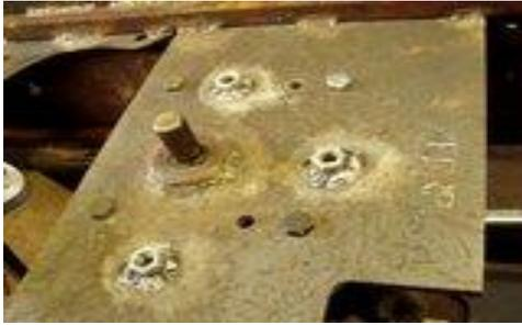
Here is a good view of the flanged nuts welded in place. The setup also makes for a fast removal setup if you are in a hurry.
