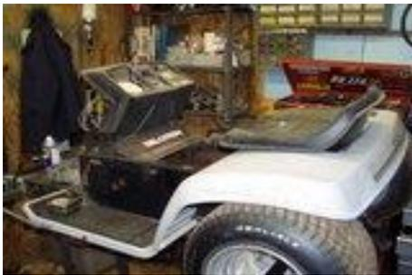
Well here is an over view of the fenders with tires on, dash slipped in place and seat on top. With this done, I can now slip the steering column in, set the steering wheel height, and finish the steering link to front axle. Dang, almost ready to slip a motor on and test it out. Hope everyone is enjoying this build.
