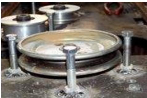
With the rear axle in and brake mounted. I am happy with all. I moved the tranny pulley belt guides while I have it all upside down. Here you can see how I do my belt guides. I weld flanged nuts to the plate and then I simply screw bolts in for my guides.
