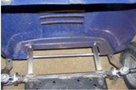
Here you can see how it sit right over the bolts. To secure it, a couple fender washers , flange nuts, and you're done.
