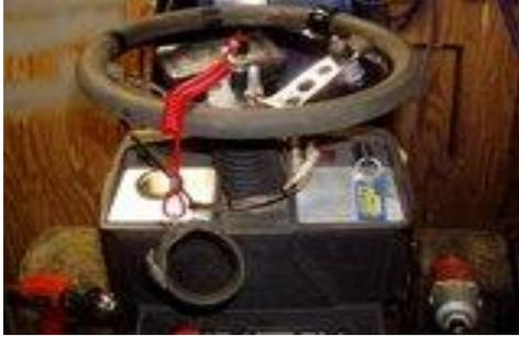
Here is a more top look at the steering wheel. 4 display digatron in top of wheel, Hand throttle just to the right of center, with starter button right there. I grab the throttle and starter button at same time with right hand while slipping the cap on the tether with left hand. Tether switch dead center. Everything is real close and easy to get to without having to look around.
