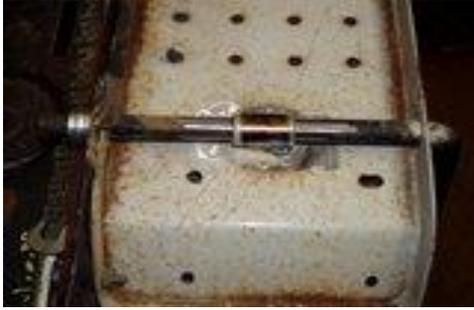
Ok here is my clutch pedal. I drilled 5/8 holes thru the side of the running board and ran the pedal thru the running board thru the frame. I used a 5/8 i.d Bushing and with it slid on the pedal welded it to the bottom of the running board. This will support it and keep a lot of the rattle previous mowers have had due to the sides of the running boards wallowing out allowing the pedal to bounce.
