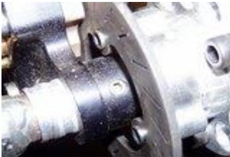
Here you see the rotor and the pins/dowels it floats on. When shimming between hub and caliper, be sure you do not shim so much. The rotor will float off the pins. This could result in a nasty ride at the end of the straight.
