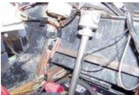
Ok here is the dash, the business end of it. You can see the small aluminum plates I made to cover the existing holes in the dash. Left side has the oil gauge and will have a second light switch for the gauge light. The right will have a volt meter, I haven't found one I like yet. That way I can just look and see if the battery is hot or needs charging.
