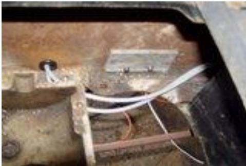
Here are the master cylinders mounted and the all lines attached.
