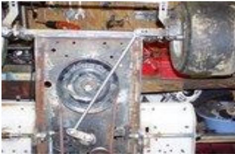
Here is an overall view of my steering set up with the E.C. Axle. I have been using this setup for going on 5 years now. I love it. 1/4, maybe a tad more, is all you will ever turn the wheel in a race.
