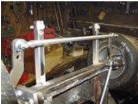
Here you see both mount welded on. Notice how I have drilled a hole, stuck a bolt in, and welded the head to the tube. Makes it easier to remove the hood and grill. Simply spin the nut off top side. You don't need two wrenches to do it.
