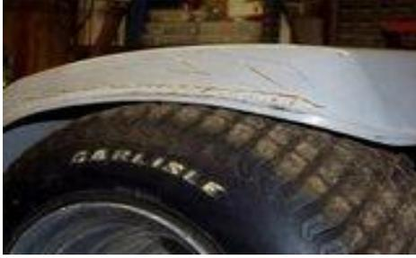
With my tallest tire on the mower (turf Masters), you see they fit and still have right at a 1/4 inch clearance. The chassis is 4-1/8 inch off the ground on the rear. And nothing has been cut.
