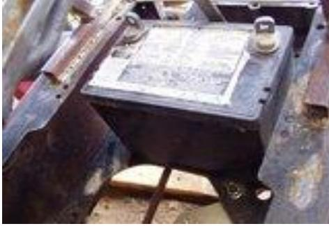
Here you see the back of the battery is up against the lip on the sub frame. Just to the right, you can see the flange nut that holds the clutch assembly.
