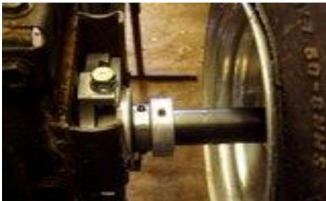
Here you can see the lock collars. E.C. sells these, and I use them outside each axle bearing like in the pic to keep axle in place, both sides of wheel hubs and both sides of brake and sprocket hubs. In this build case the brake hub is against the bearing hub so it only required one side. A total of 9 on this setup where I usually use 10.
