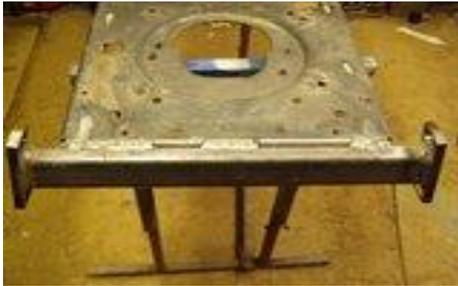
Front beam welded in place and ready to start front end assembly.
