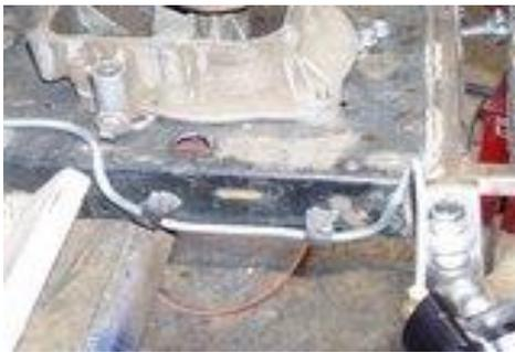
It also runs up and inside the frame around to the right side behind the steering column in front of the battery. Again extra protection of the lines.
