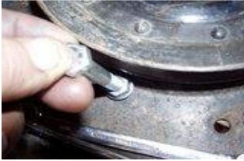
Ok here is the placement of my front pulley guides. I hold it right up against the pulley without touching it. Tack the flanged nut in place. I do this to all three, then remove the bolts and pulley and weld them on solid. This makes for a fast guide removal to change belts quickly if needed.
