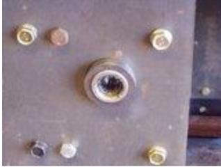
As you can see it aligns perfectly. Now tack it in place and then remove the tranny case and weld it completely in.
