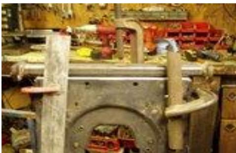
Since I am getting so much done in a short amount of time, I decided before I quit I will mount the front axle beam. I clamp two straight edges to the top of the frame I pull the axle up to it and center it equally side to side and clamp it in place.
