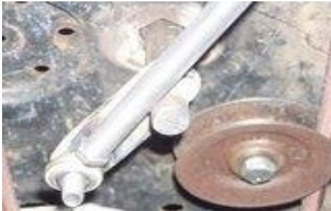
Here you can see how I gauge where to cut the shaft off at. I leave it long enough so it serves as a stop at full right turn. I don't have a stop for left turn. I have never went over. The tire hits the grill before it does, so it serves as a stop. I don't use the left turn much. Now the right in counter steering, yea I sometimes hit full lock.
