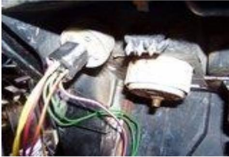
I run the wires for the starter button and kill switch up through the boot that covers the steering column, above the dash, thru a hole I drill in the steering wheel, then over to the starter button, and kill switch in center of wheel.
