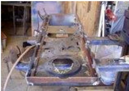
Ok here's the rails and tranny plate from the bottom all done and welded in.
