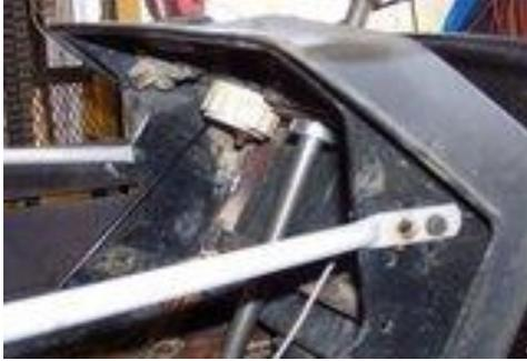
Here are the grill support rods bolted to the dash, and the bar I weld in. I drill and tap for 1/4 threads, then simply run a bolt in, no nut. Makes for quick removal.
