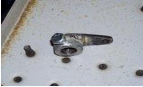
Here is my rod mount for my clutch pedal. I make the arm then weld it to the 5/8 lock collar. I then slip it over the end of the pedal and use a bolt instead of the set screw to lock it down. I drill into the pedal and tap it so that I am screwing not only thru the collar but into the pedal also. Makes for a sure tight fit.
