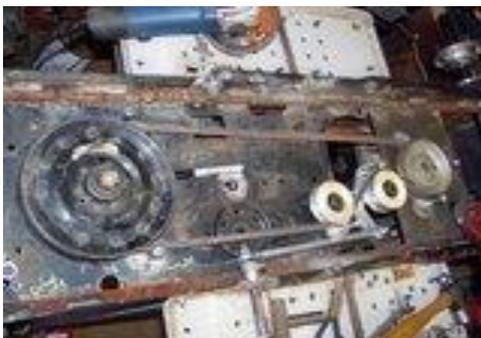
Here is the clutch assembly completed, rod in place. Next I will show you how I do the guides for the motor pulley.
